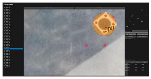
If you mismark the position of the ground control point, click Clear all marks button and reselect. Otherwise, click Confirm unknown marks. A useful tool for checking the appropriation of GCPs are their residuals. If displacements of selected points are high, you should check if you forgot to survey one of them (their position is missing in the file). Described method of Automatic orientation as furtherly described Troubleshooting with orientation in chapter *Troubleshooting with orientation*.
