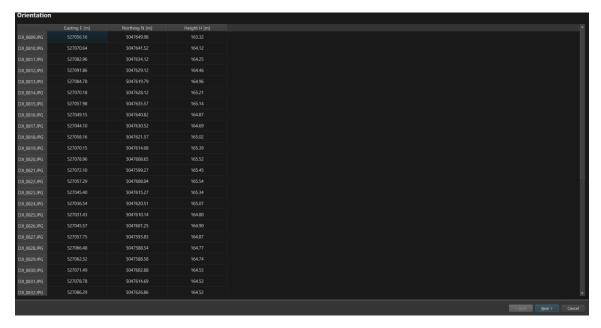
Orientation summary window presents residuals of adjusted camera positions on all three axis and its spatial value. Click Finish to complete orientation. If some images have errors in telemetry, they appear as unregistered in the List of images in Working panel.
