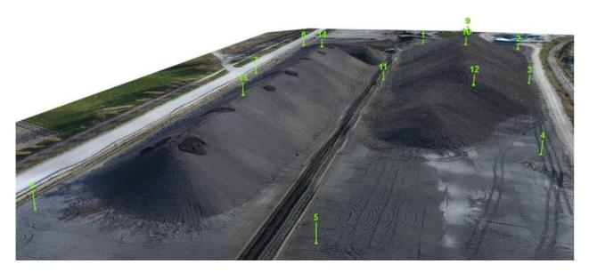
To achieve survey-grade accuracy, place your GCPs 50-100 m apart. Higher density of GCPs also means higher accuracy of end results.
