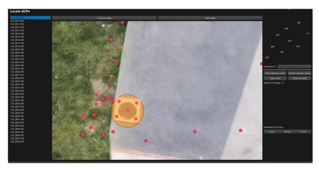
Continue by selecting additional two GCPs from other segments of your project area. When you select the third ground control point the automatic recognition for all other GCPs will start. Three marked GCPs remain orange coloured while automatically found GCPs are now coloured green and the names of all GCPs are identified.
