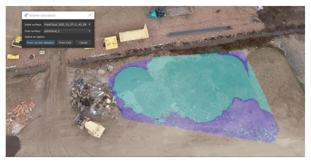
Use a CAD .dxf file as a contour. To calculate the volume of the area defined by the .dxf boundary, click Calculate Volume. For the initial surface, select the initial surface. For the final surface, select the final surface. Click From CAD and open the desired file.
