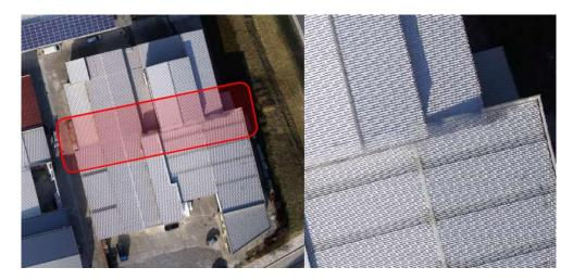
To eliminate the over-the-building image stitching we advise you to have the whole building on a single image. First, perform your mission at 80 m AGL, then manually trigger a few nadir images from a higher AGL (120 m above the object, for example) to get the whole object in one image. That enables you to recalculate the area with - or/and around - the building.
