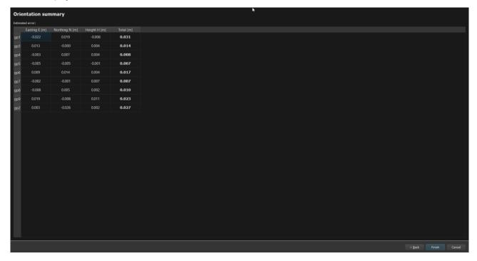
To check for independent accuracy quality, GCPs can be marked as Validation points that provide independent values to compare against GCP values. Points defined as Validation points get coloured grey.
