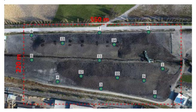
In case of uneven (or rugged) terrain it is highly recommended to place GCPs on both lowest and highest points of your area of interest.
