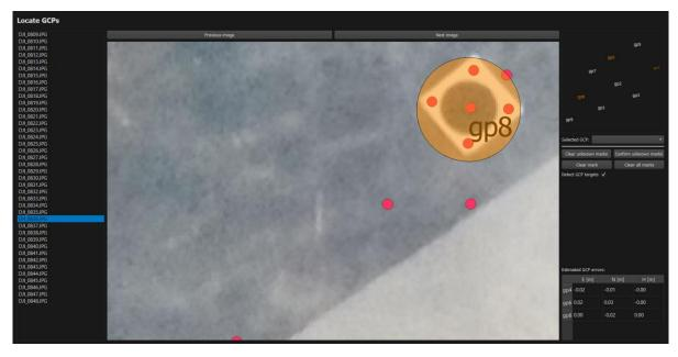
In the lower right corner appears the **residuals** of marked points. Residuals should be within 1m. Check if the automatic positions are calculated correctly - GCPs need to be coloured green. If not, correct them with manual selection. First, select the name of GCP on GCP map, then show the exact position of GCP map on an image. Use left mouse click.
